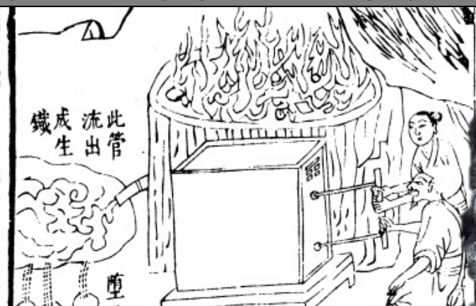
1648 CHINESE ILLUSTRATION OF SMELTING IRON ORE TO MAKE WROUGHT IRON
